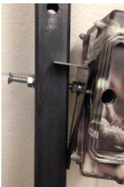
**Figure 6.** Custom L-bracket attached between the post and camera to adjust the tilt of the unit.
