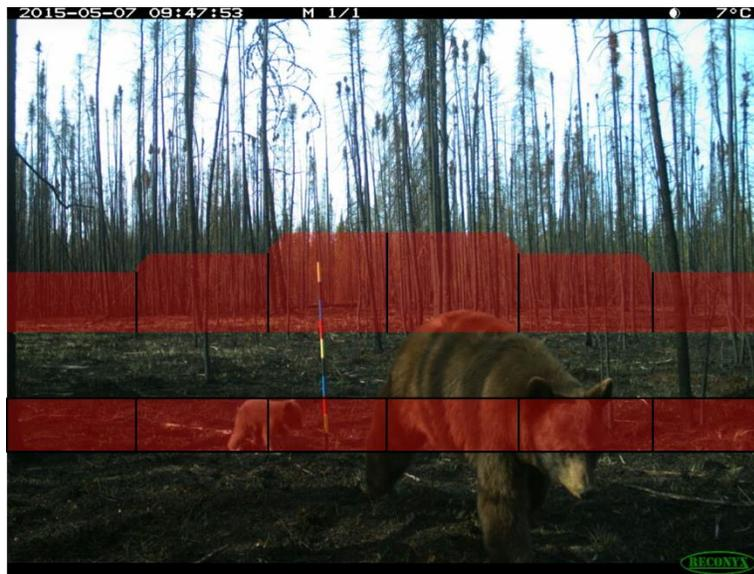
**Figure 4.** Remote camera detection bands, relative to the location of the painted conduit.
