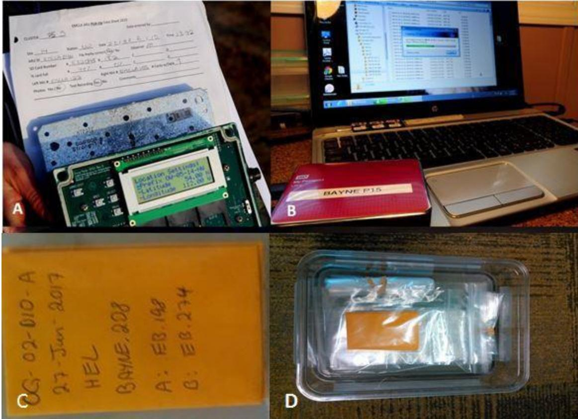
Figure 2. Down-loading data. A. Check file prefix on ARU against the data sheet and cross reference using ARU number. B. Copy data from SD card onto back-up hard drive. C. Put SD card into labelled envelop. D. Store cards with data in a clearly labelled secure container and put all cards from each site into individual Ziploc bags.
